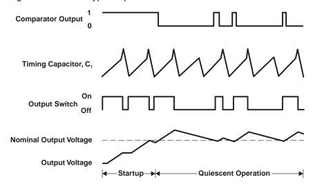
**Figure 5. Typical Operation Waveforms**
