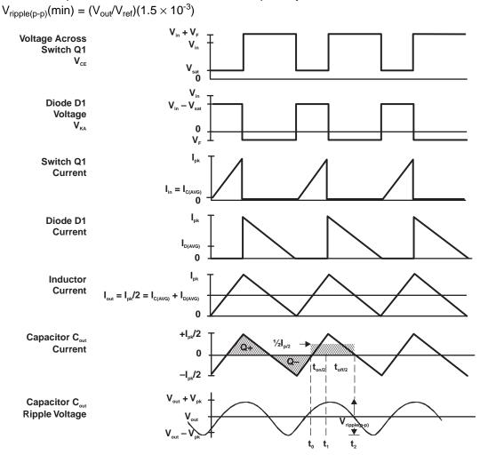
Figure 7. Buck Switching Regulator Waveforms
