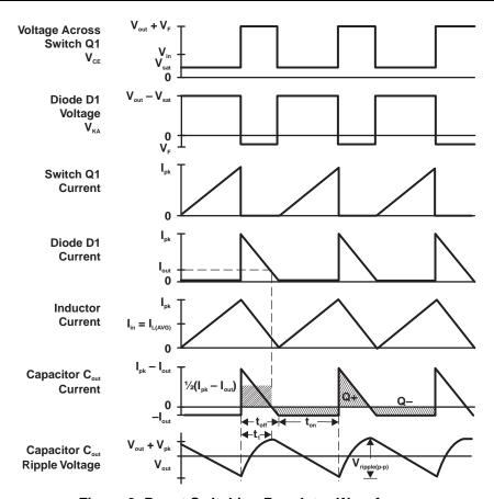
Figure 9. Boost Switching Regulator Waveforms
