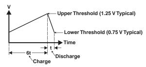
Figure 3. Oscillator Voltage Thresholds
