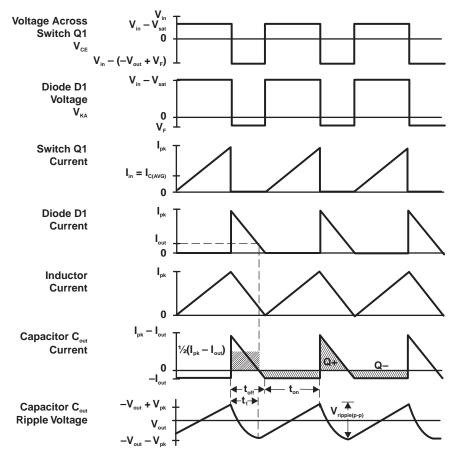
Figure 11. Inverter Switching Regulator Waveforms
