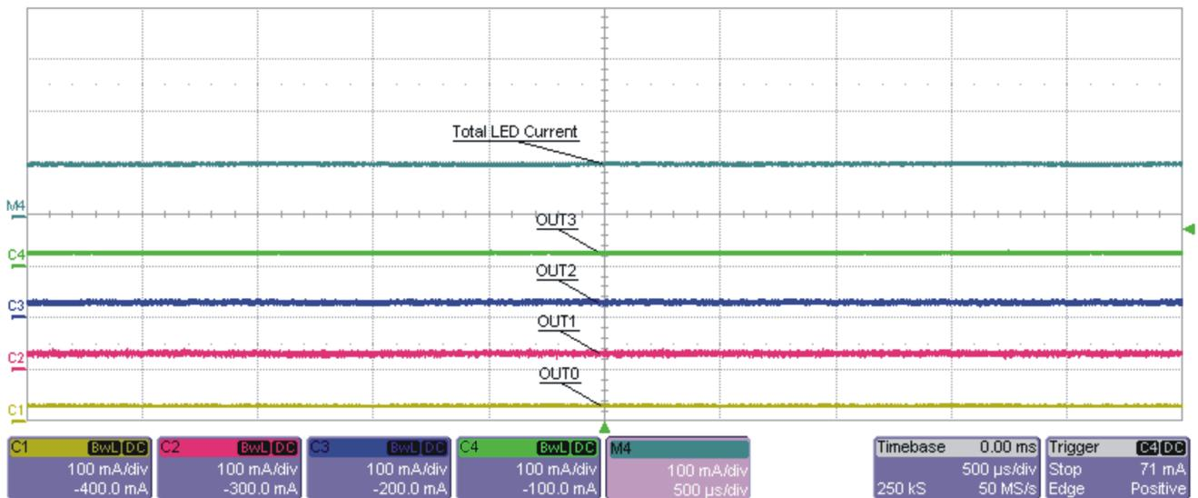
**Figure 3. LED Programmed to 30% Brightness**
