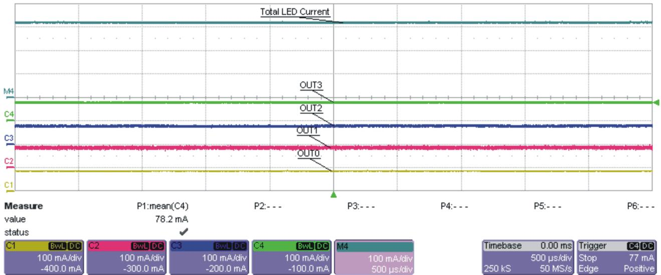
**Figure 2. TLC5922/23/24 Output Current and Total Current Through D1**
