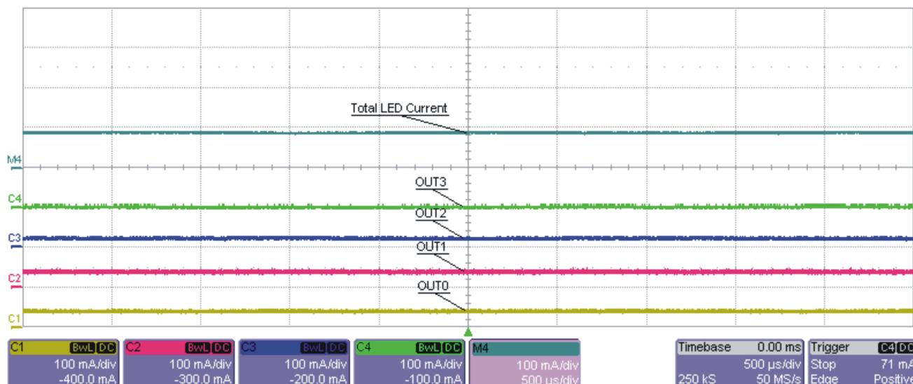
**Figure 4. 30% Analog Dimming — Unequal Output Currents**
