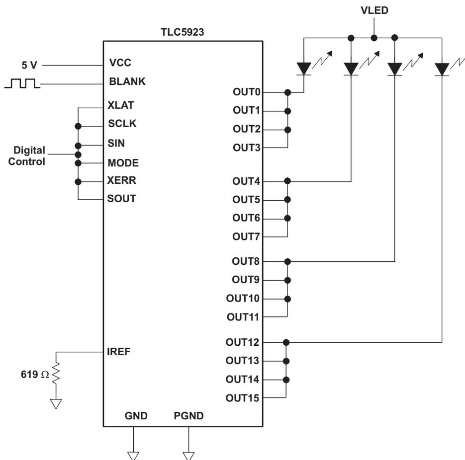
**Figure 1. TLC5922/23/24 Configuration Driving Four White LEDs**
