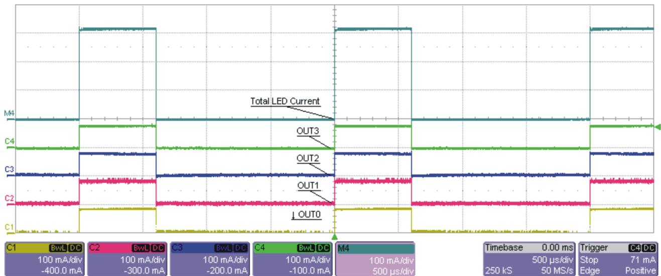
**Figure 5. 30% PWM Dimming — 500 Hz**
