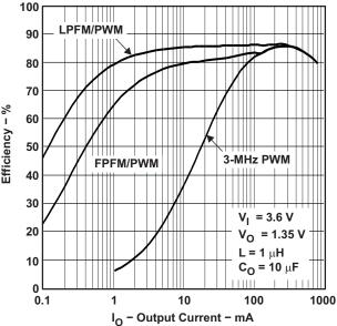
Figure 6. Efficiency vs Output Current
