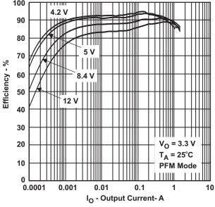
Figure 5. Efficiency vs Output Current
