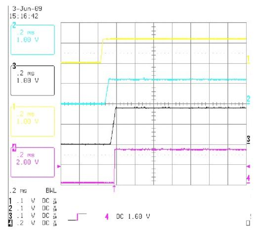
Figure 3. Sequencing in Start-up Waveform
