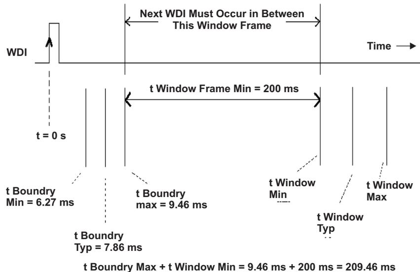
**Figure 1. For the Case Where  $WDT = WDR = 0\text{ V}$  (TPS3813)**
