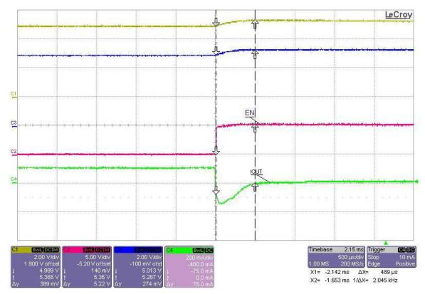
Figure 4. Time Between Fault and Zero Current
