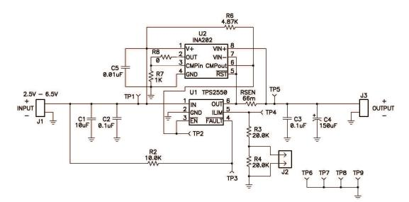
Figure 1. USB Power Switch Schematic with Reverse Current Protection
