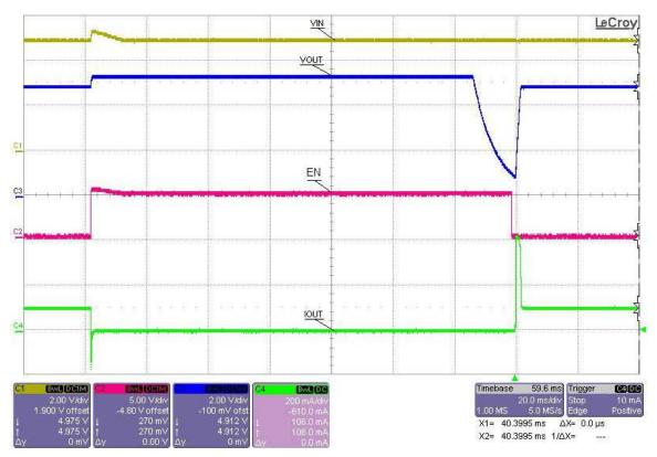
Figure 2. Responding to Reverse Current
