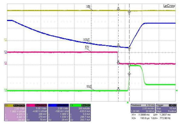
Figure 5. Unlatching When Output Decays
