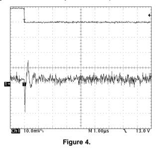
With 1 nF capacitive load, the output is stable and the transient ringing falls into the noise floor.
