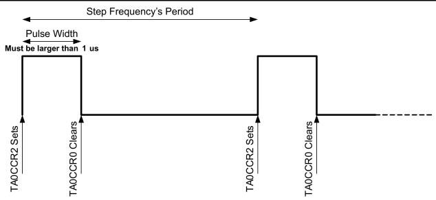
Figure 2-2. Timer A0 Used to Generate STEP Pulses
