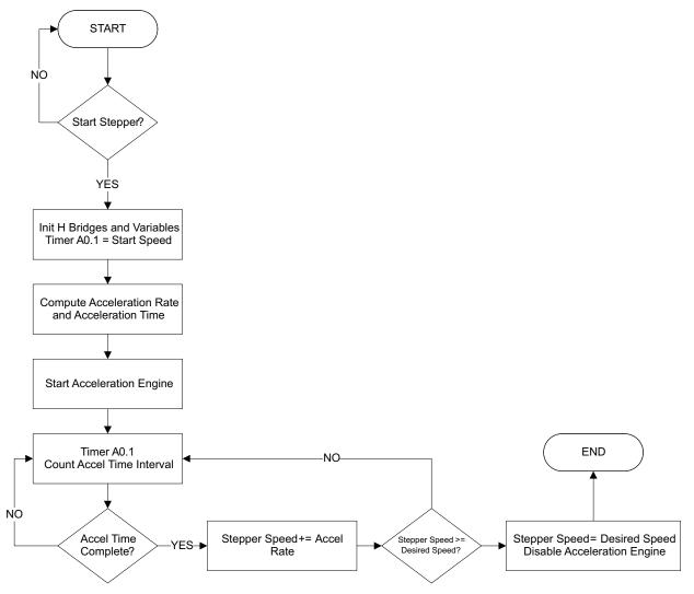
Figure 2-4. Stepper Speed Acceleration Flowchart
