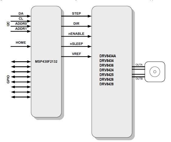
Figure 1-2. Intelligent Stepper Controller Block Diagram
