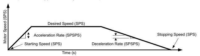
Figure 2-1. Typical Stepper Acceleration and Deceleration Profile
