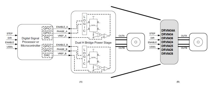
Figure 1-1. Stepper Control Logic and Power Stage
