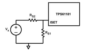
Figure 1. TPS61181 Analog Dimming Configuration
