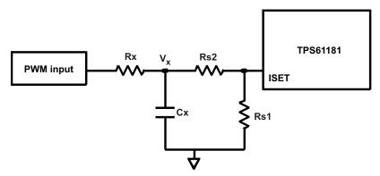
Figure 2. RC Filter to get the Average Value of PWM Signal
