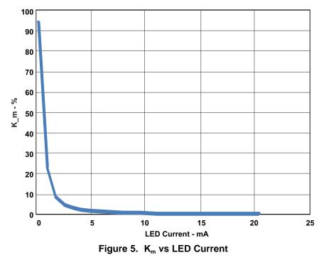
If it is necessary to operate at these low current levels it is advisable to use the traditional built-in PWM dimming scheme, either in conjunction with analog dimming or by itself. If PWM dimming causes the LED current to switch between 0 and 5 mA, instead of between 0 and  $I_{LED(max)}$  (20 mA in this example), the EMI noise disruption would be significantly less than if the PWM dimming scheme was used for the entire current range.
