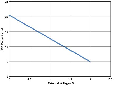
Figure 3. Theoretical Led Current and External Voltage
