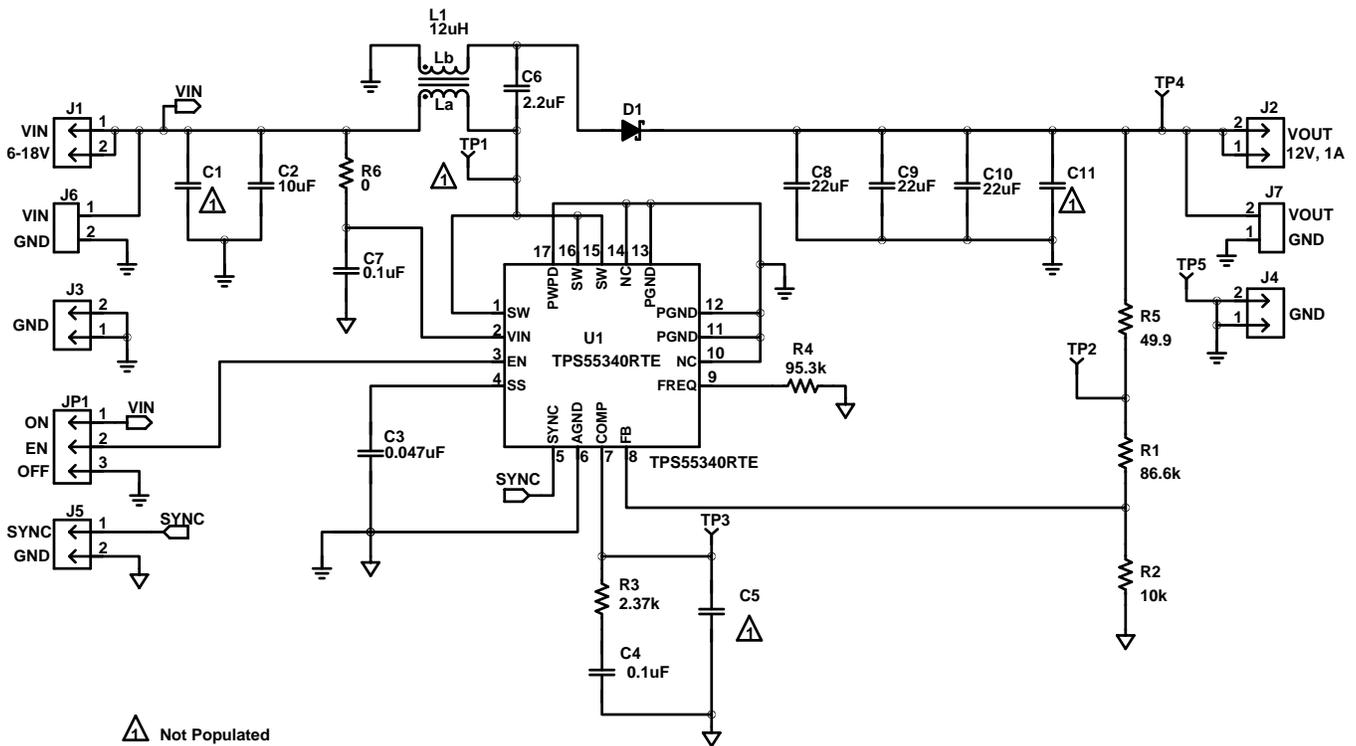
Figure 4. TPS55340EVM-147 Schematic
