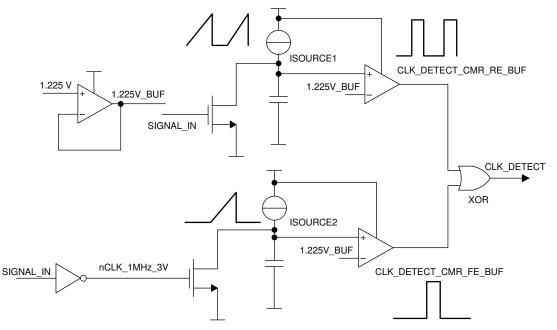
Figure 5-7. Loss-of-Clock Monitor
