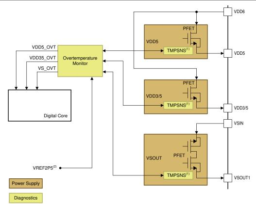
(1) Temperature sense elements are placed close to the power-FETs (PFETs) of the corresponding power supplies.
