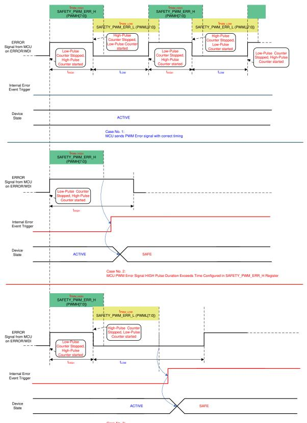
Case No. 3: MCU PWM Error Signal LOW Pulse Duration Exceeds Time Configured in SAFETY\_PWM\_ERR\_L Register
