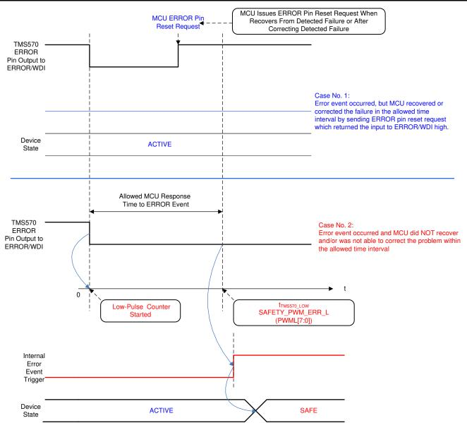
Figure 5-2. Error Detection Case Scenarios in TMS570 Mode
