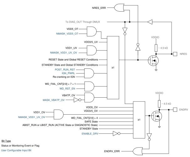
Figure 4-2. Reset (NRES) and Enable (ENDRV) Circuit
