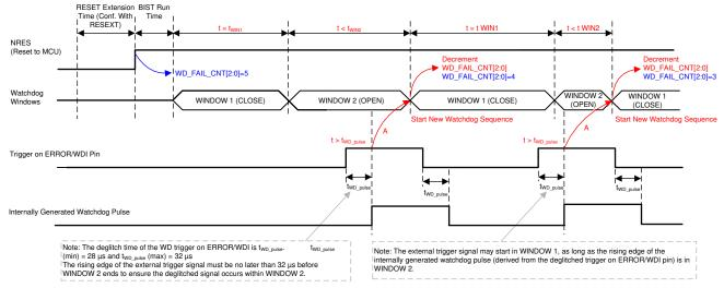
A. When a *good event* is received in Window 2 (OPEN), 1 system clock-cycle (250 ns, typical) later the next watchdog sequence begins. Therefore the actual length of Window 2 (OPEN) depends on when the MCU sends the good event.
