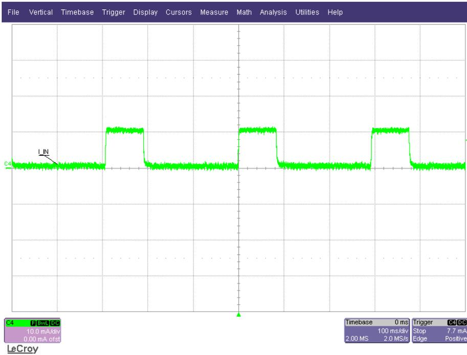
Figure 8. Input Current in Sleep Mode with MODE Low ( $I_{LED} = 0 \text{ mA}$ )
