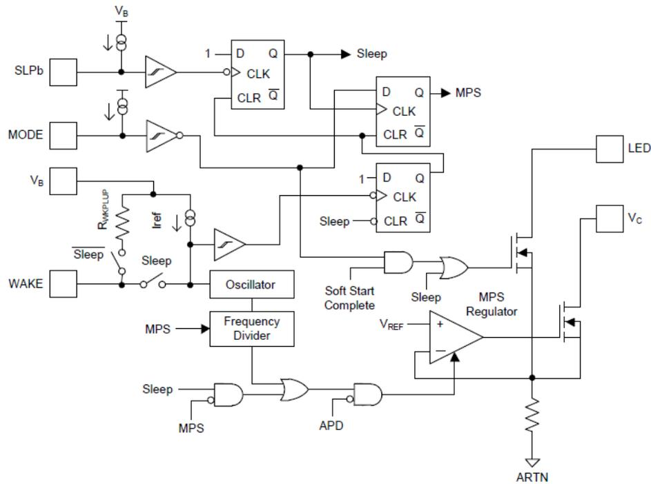
**Figure 1. TPS23752 Sleep Mode Functionality Block Diagram**
