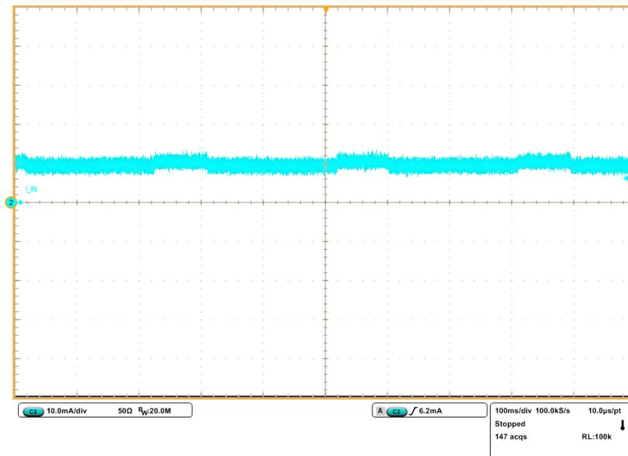
**Figure 13. Input Current in Sleep Mode with MODE Low ( $I_{LED} = 9.081$  mA)**
