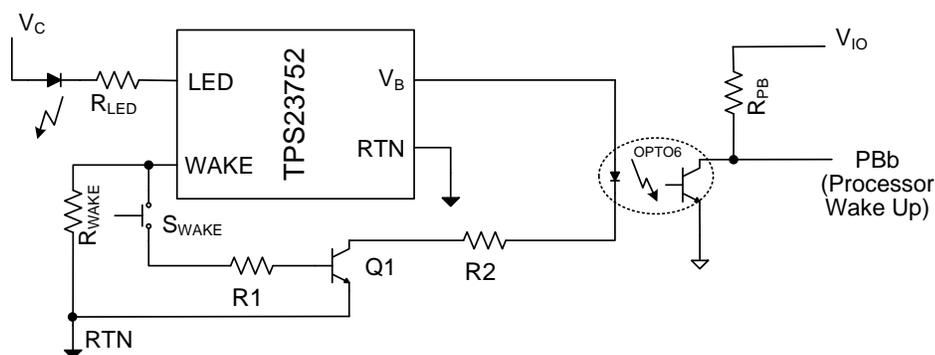
**Figure 4. WAKE Pin Connection with Low CTR Optocoupler**
