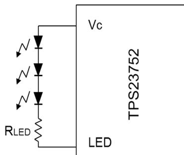
**Figure 3. LEDs Connection For Higher Brightness**
