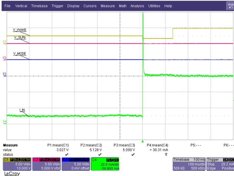
Figure 12. Exiting Sleep Mode with MODE High and SLPb High
