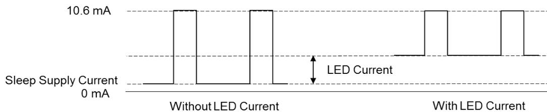
**Figure 2. TPS23752 Pulsed MPS Current in Sleep Mode**
