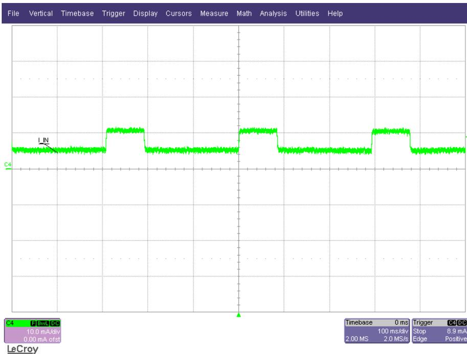
Figure 9. Input Current in Sleep Mode with MODE Low ( $I_{LED} = 4 \text{ mA}$ )
