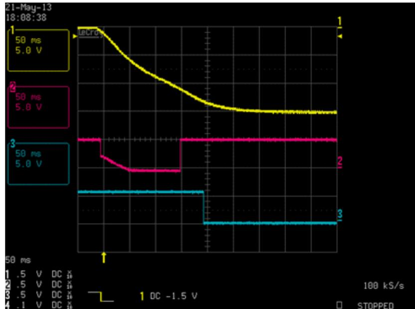
Figure 5. OUTA and OUTB Response for VDD Voltage Rising
