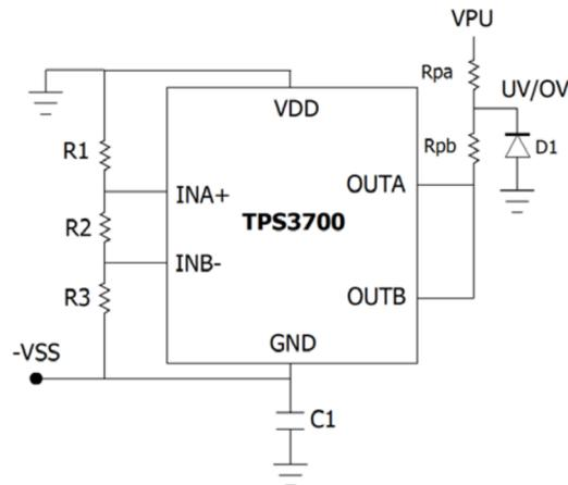
Figure 3. Wired-OR Output Configuration
