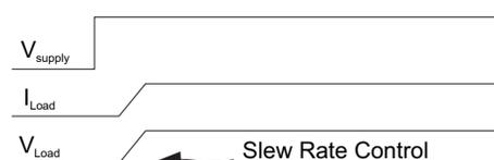
Figure 7. Slew Rate Control with Load Switch
