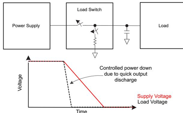
Figure 9. Controlled Power Down with Load Switch
