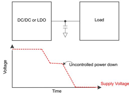
Figure 8. Uncontrolled Power Down without Load Switch
