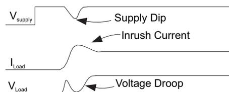
Figure 6. Inrush Current Causing Power Supply Dip
