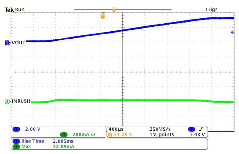
Figure 12. TPS22965 Scope Capture (CT cap = 2200 pF)
