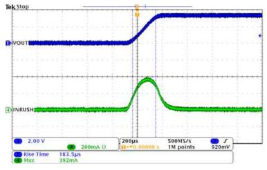
Figure 7. TPS22902B Inrush Current
