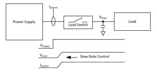
Figure 6. Typical Load Switch Application Circuit
