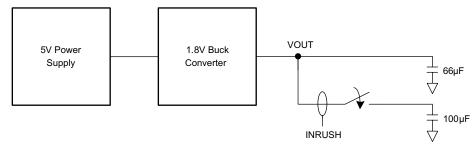
Figure 13. System Block Diagram without Slew Rate Control
