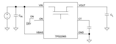
Figure 8. TPS22965 Application Circuit
