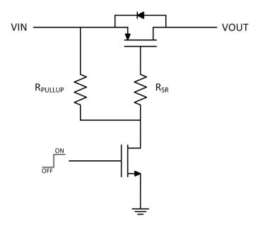
Figure 5. Discrete Load Switch Implementation
