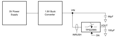
Figure 15. System Block Diagram utilizing the TPS22965
