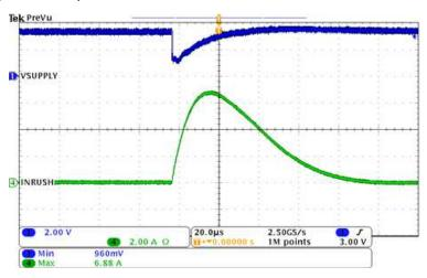
Figure 4. Power Supply Dip due to Inrush Current
