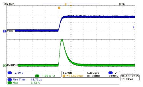
Figure 2. 3.3V Applied to a 47µF Capacitor
