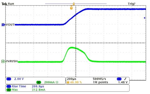
Figure 11. TPS22965 Scope Capture (CT cap = 150 pF)
