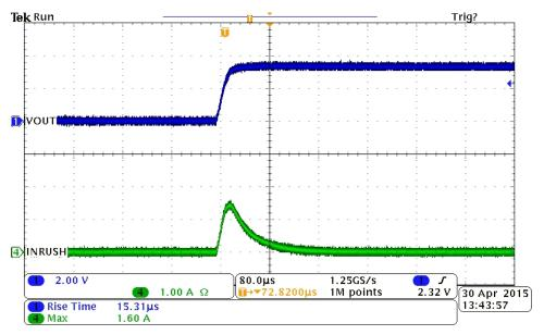
Figure 3. 3.3 V Applied to a 22 µF Capacitor
