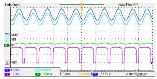
Figure 3. VGS Drops With Low IOUT (48 mA) and Noisy Input Voltage
