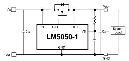
Figure 1. LM5050-1 Application Circuit
