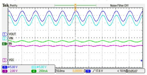
Figure 4. Stable VGS With 1-µF Input Capacitor and 0.1-µF Output Capacitor
