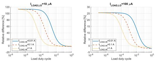
Figure 2-1. Relative Difference in Battery Consumption vs Load Duty Cycle
