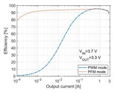
Figure 1-2. TPS63805 Efficiency vs Output Current
