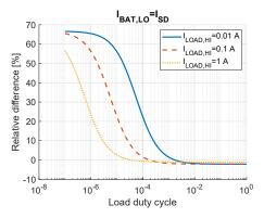
Figure 2-2. Relative Difference in Battery Consumption vs Load Duty Cycle
