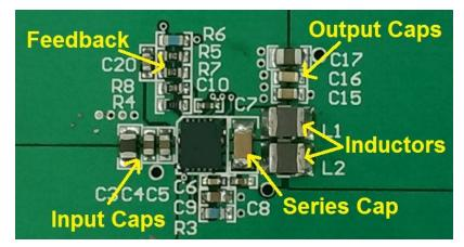
Figure 14. Series Capacitor Buck Converter Prototype Using TPS54A20
