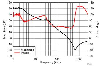
Figure 19. Bode Plot Showing Magnitude and Phase
