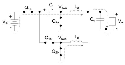
Figure 5. Interval 1: Phase A High Side Switch (Q1a) on
