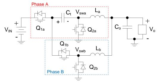
Figure 1. Two-phase Series Capacitor Buck Converter
