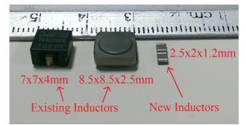
Figure 2. Inductor Size Comparison for a 10-A Application
