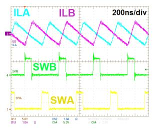
Figure 15. Steady-State Series Capacitor Buck Converter Waveforms
