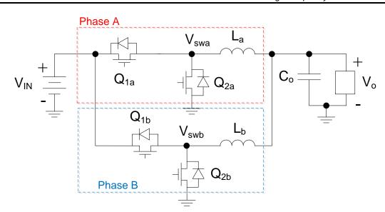
Figure 3. Two-phase Buck Converter
