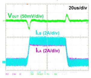
Figure 18. Load Transient Response
