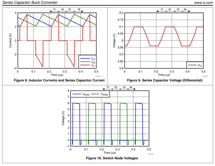
The main differences between the series capacitor buck converter and the conventional buck converter are that the duty ratio of the high side switches is doubled, switching occurs with half the drain-to-source voltage experienced by switches in a buck converter, inductor current balancing is automatic, and inductor current ripple is decreased. All these factors are favorable for high frequency and high conversion ratio converters.
