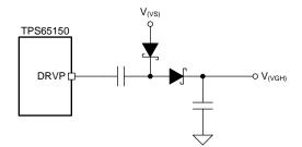
Figure 3. One-Stage Positive Charge-Pump Circuit
