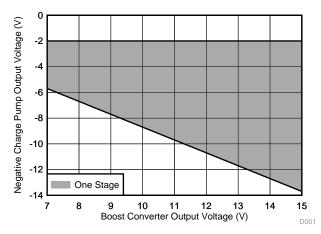
Figure 2. Negative Charge-Pump Output Voltage Range
