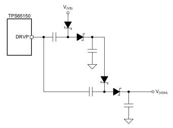
Figure 4. Two-Stage Positive Charge-Pump Circuit
