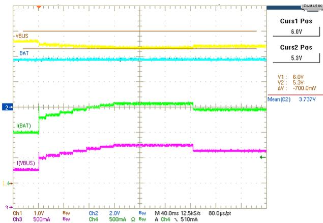
Figure 3. Automatic ICO Detection After Charge Current Increase With  $V(BAT) > V_{MINSYS}$
