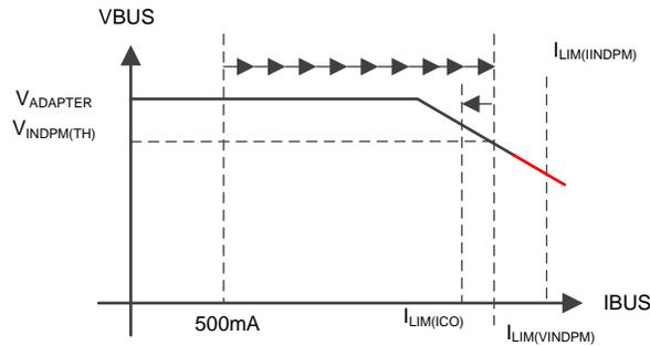
Figure 2. Graphical Representation of ICO During Operation
