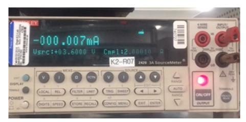
Figure 6. Reduced Leakage Current Confirmed with Keithley Sourcemeter
