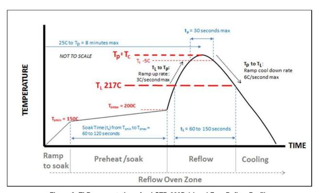
Figure 3. TI Representation of a J-STD-020D.1 Lead-Free Reflow Profile
