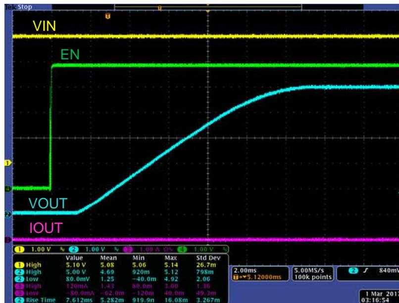
Figure 6. Soft Start Behavior With No Load
