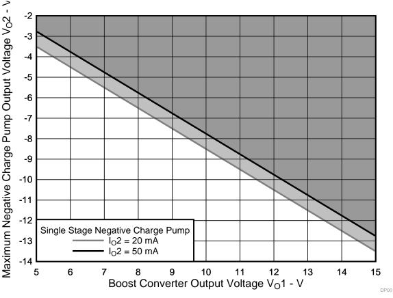
Figure 2. Negative Charge-Pump Output Voltage Range
