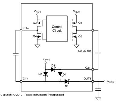
Figure 4. Tripler Positive Charge-Pump Circuit
