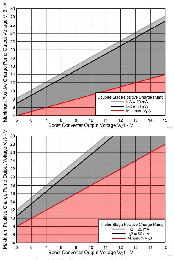
How to Estimate the Output Voltage Ranges of the Charge Pumps in the TPS6510x and TPS6514x Devices Copyright © 2017, Texas Instruments Incorporated
