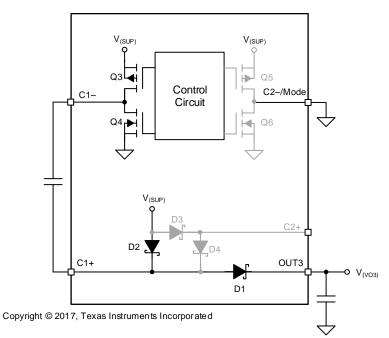
Figure 3. Positive Charge-Pump Circuit in Doubler Mode
