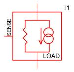
Figure 3. DVM Load Graphic From SiMetrix
