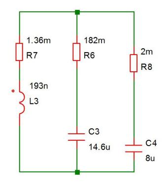
Figure 14. Three-Branch Lumped Model Screen Capture From SiMetrix
