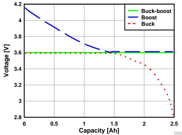
Figure 2. Voltage Obtained from Li-ion Battery Using Different Topologies
