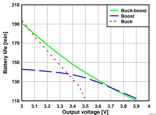
Figure 4. Battery Lifetime vs. Output Voltage: Resistive Load (3.6 Ω)
