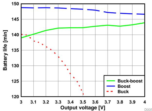
Figure 5. Battery Lifetime vs. Output Voltage: Constant Power Load (3.6 W)
