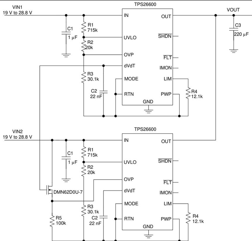
**Figure 3-4. Semi-Integrated Power MUX using 2x TPS2660 eFuses**
