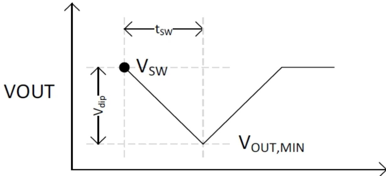
**Figure 4-1. Voltage Dip on Output During Switchover Time**
