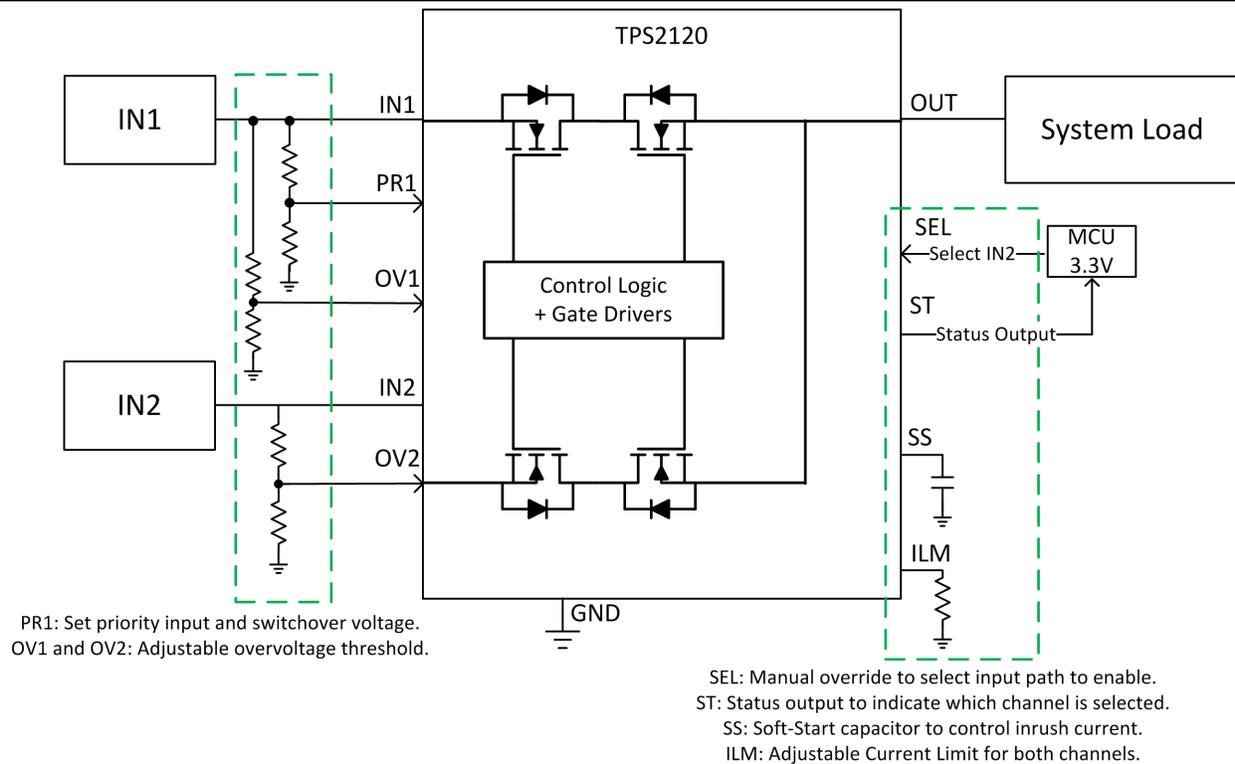
Figure 3-5. Fully-Integrated Priority Power MUX with TPS2120
