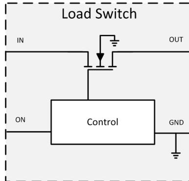
**Figure 3-2. Load Switch with Parasitic Body Diode Removed**
