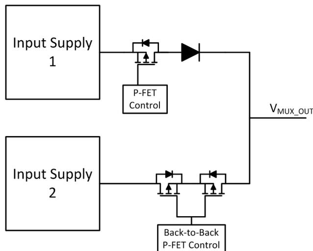
**Figure 1-3. Example Priority Power MUX**
