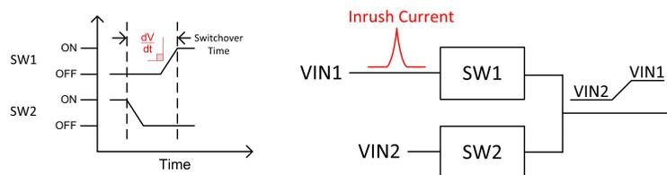
**Figure 4-2. Inrush Current Spike Caused by Supply Switchover**
