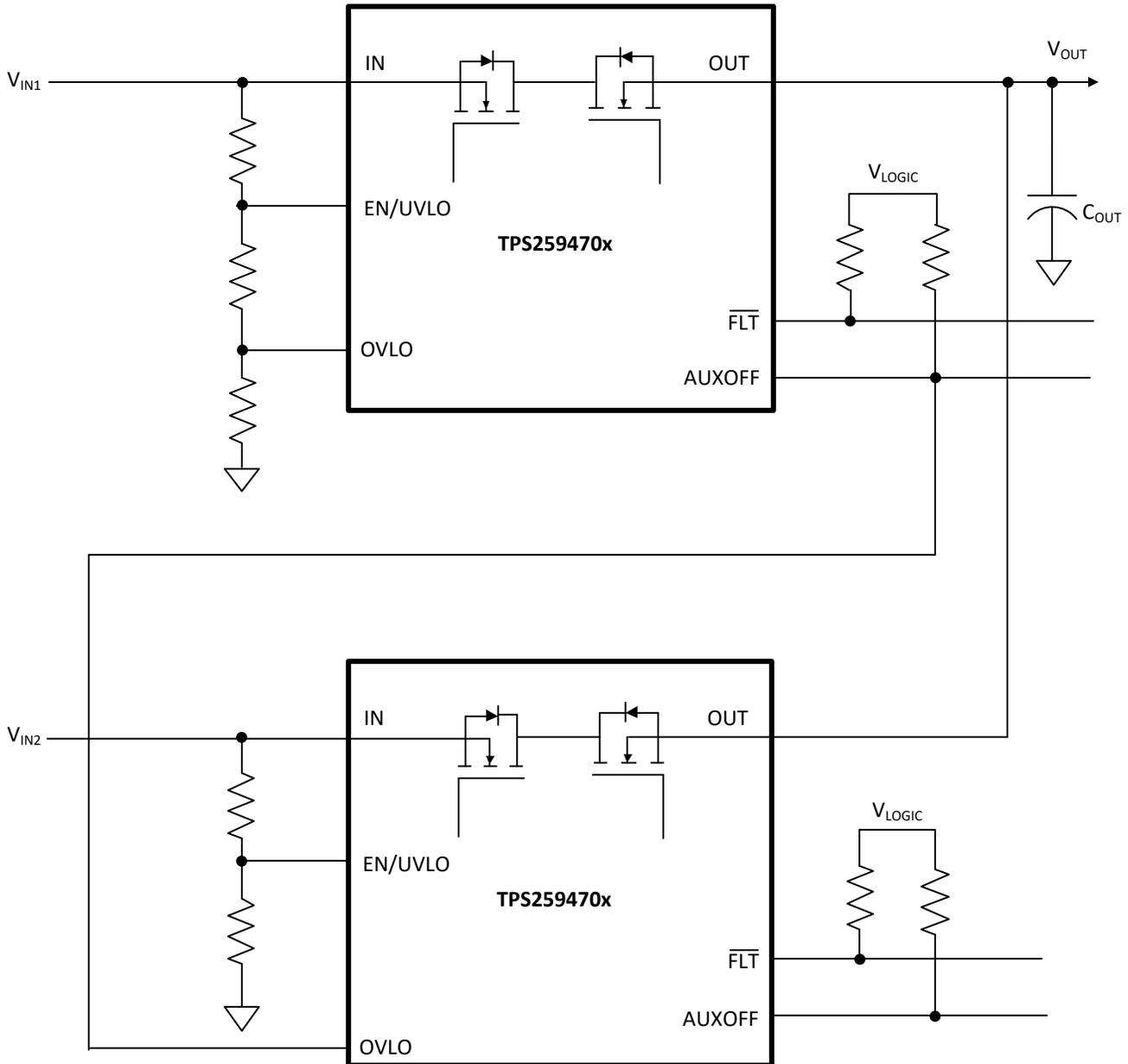
Figure 2-2. Automatic Power MUX using 2x TPS259470x eFuses
