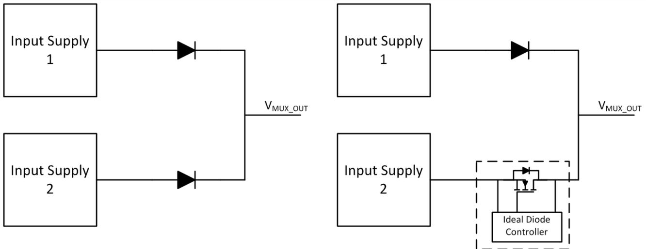
**Figure 1-2. Minimum Functionality for Power MUX Without Priority**
