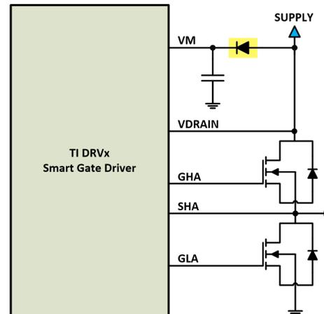
Figure 1. Modified Circuit with Diode
