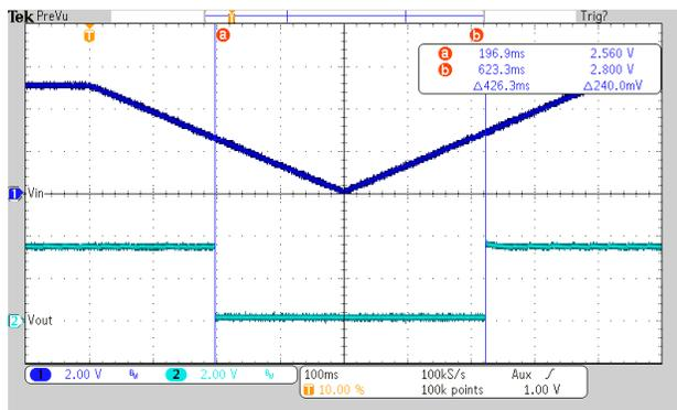
**Figure 2. Achieved cutoff and turn-on input voltage thresholds**
