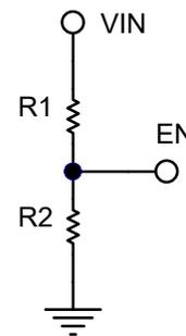
**Figure 1. Setting the input cutoff voltage with a voltage divider**
