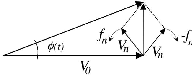
**Fig. 3.** Phasor-plane representation of the carrier affected by the two side tones responsible for sole phase modulation
