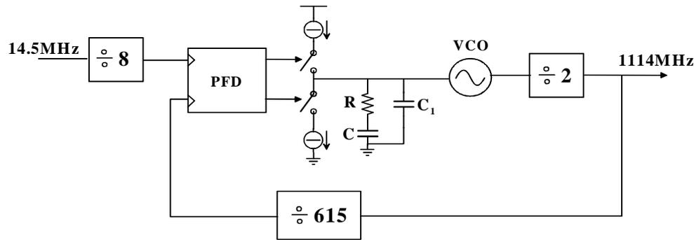
Fig. 6. Scheme of principle for the integrated phase-locked loop used in the experimental validation
