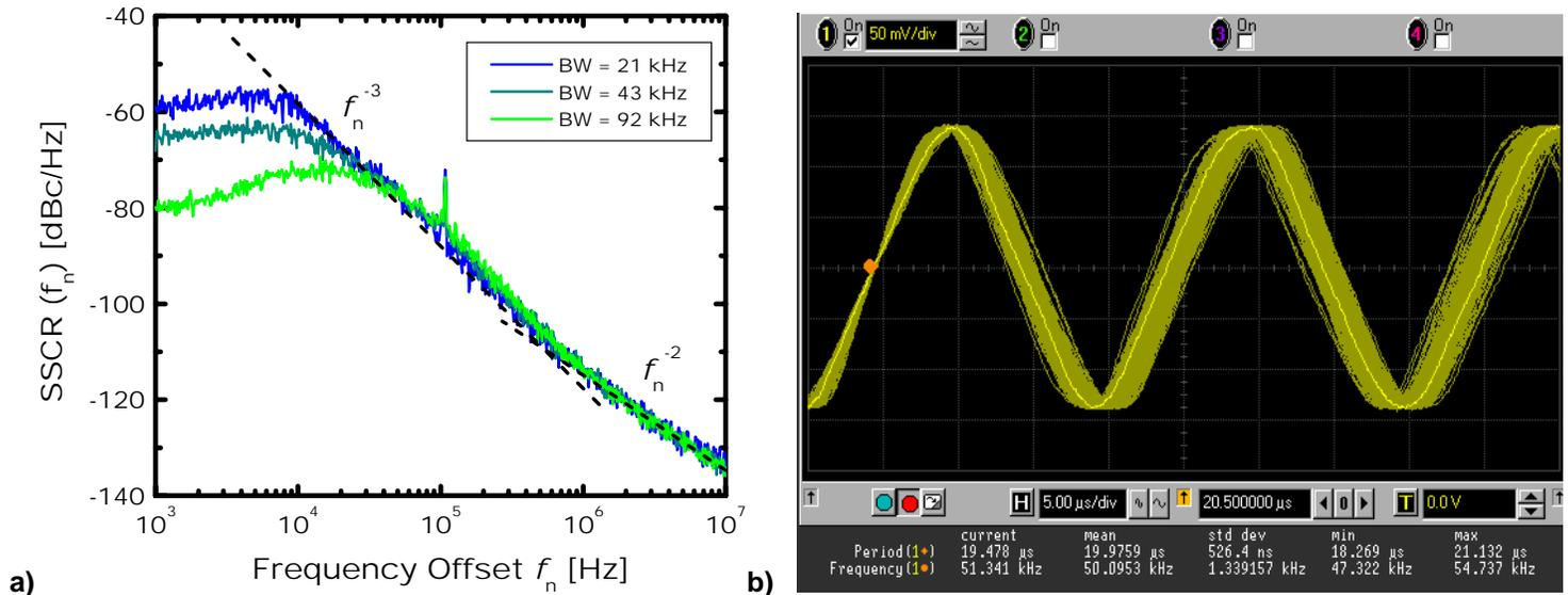
**Fig. 7.** a) Experimental SSCR plots for the CMOS PLL frequency synthesizer operated with different bandwidths. b) The jittering zero-crossings of the PLL output, as captured with an Agilent Infiniium™ oscilloscope
