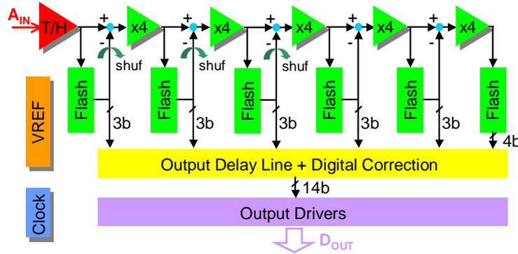
Fig. 8. Pipelined converter architecture (2.5 bit per stage), with integrated internal references and on-chip clock driver
