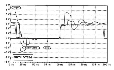
Figure 21. Waveforms on an Open-Circuit Line
