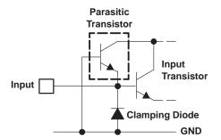
Figure 16. Input Circuit With Parasitic Transistor
