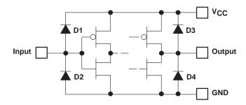
Figure 11. ESD-Protection Circuits Using Diodes
