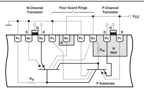
Figure 3. Guard Rings in a CMOS Circuit
