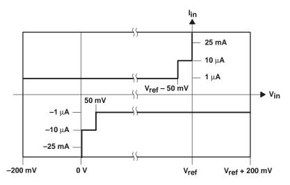
Figure 18. Characteristics of Voltage Limiter TL7726
