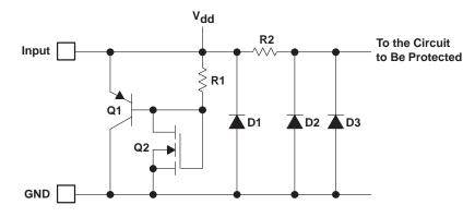
Figure 12. Two-Stage ESD-Protection Circuits
