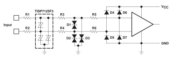
Figure 14. Protection Circuit for Extreme Requirements
