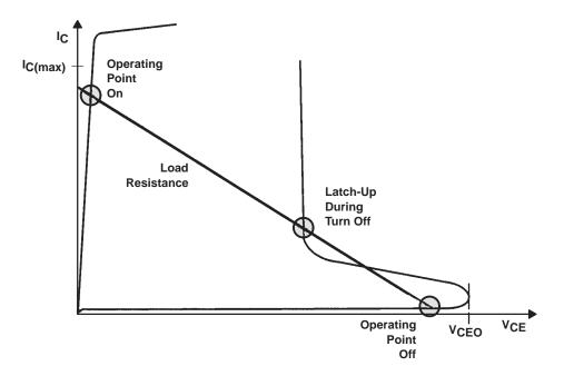
Figure 6. Output Characteristics With Load Resistor
