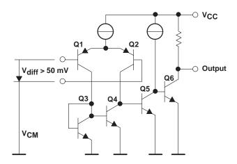
Figure 5. Simplified Circuit of a Differential Amplifier
