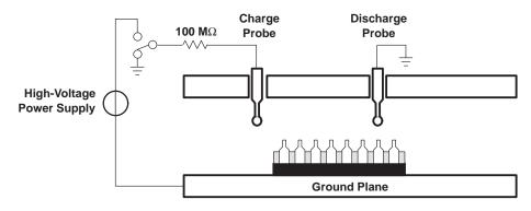
Figure 10. Charged-Device Model Test Setup
