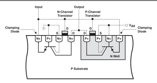
Figure 17. Parasitic Transistors in CMOS Circuits
