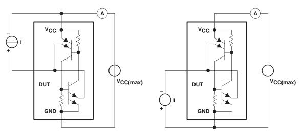
Figure 4. Latch-Up Test Circuit
