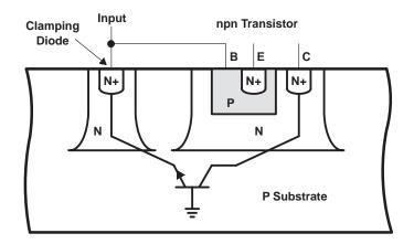
Figure 15. Parasitic Transistors in Bipolar Circuits
