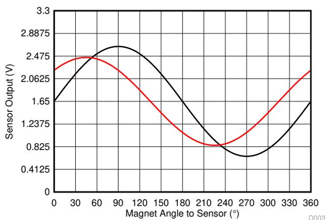
Figure 4-7. Two Sensors  $45^\circ$  Apart Uncalibrated Data
