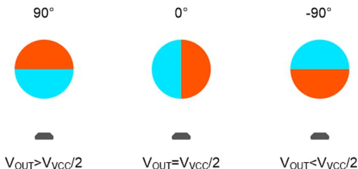
**Figure 4-1. Uncalibrated Sensor Positions**
