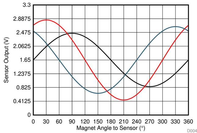
Figure 4-9. Three Sensors 60° Apart Uncalibrated Data
