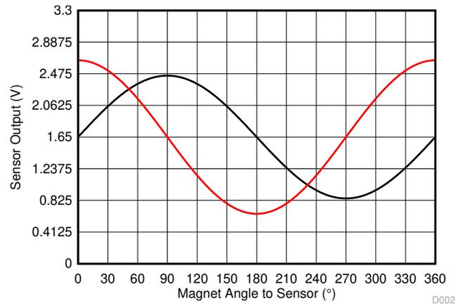
Figure 4-5. Two Sensors 90° Apart Uncalibrated Data
