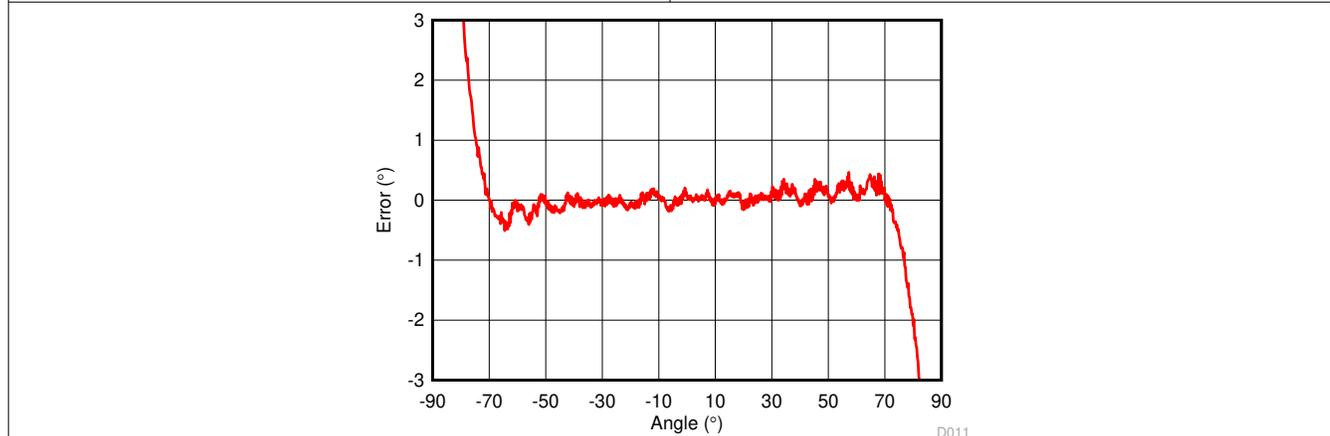
**Figure 4-16. One Sensor Lookup Table Calibrated Error, 16 Cal Points,  $\approx 1^\circ$  Peak-to-Peak Error**
