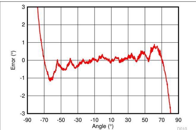
**Figure 4-15. One Sensor Lookup Table Calibrated Error, 10 Cal Points,  $\approx 2^\circ$  Peak-to-Peak Error**
