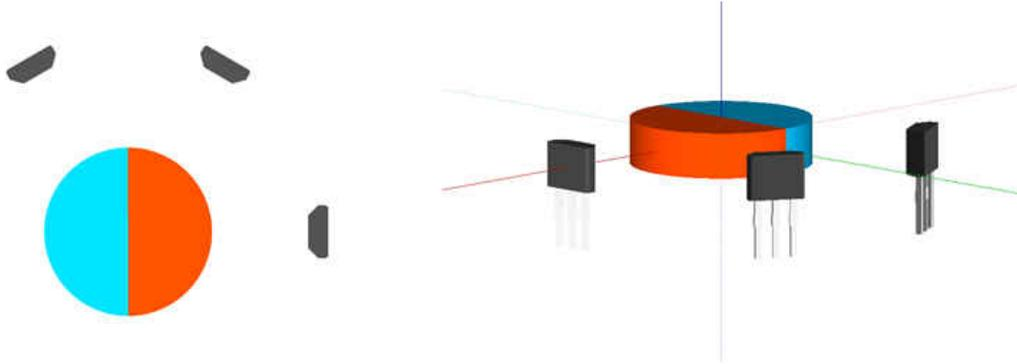
Figure 4-8. Three Sensors 60° Apart
