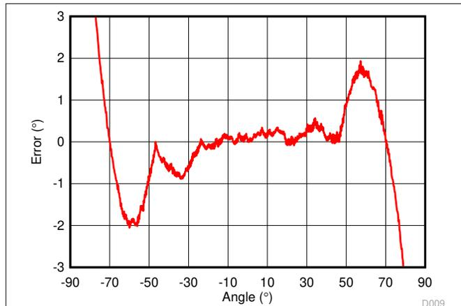
**Figure 4-14. One Sensor Lookup Table Calibrated Error, 7 Cal Points,  $\approx 4^\circ$  Peak-to-Peak Error**
