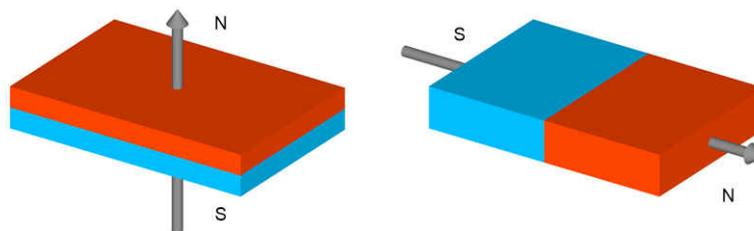
**Figure 2-3. Block Magnets**
