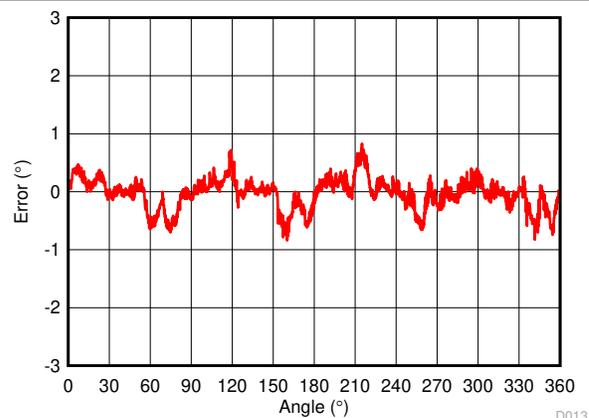
Figure 4-18. Two Sensors Lookup Table Calibrated Error, 26 Cal Points,  $\approx 2^\circ$  Peak-to-Peak Error
