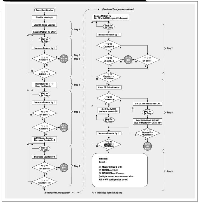
MasterID. The MasterID is compared with AIC10Num-1. If they are not equal to each other, the IdentFail flag is set, an alarm sounds, and the system aborts to reset condition.
