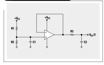
connected to V<sub>CC</sub>+, and ground is connected to V<sub>CC</sub>- or GND. A virtual ground, halfway between the positive supply voltage and ground, is the "ground" reference for the input and output voltages. Voltage swings above and below this virtual ground to V<sub>OM</sub>±. Some newer op amps have different high- and low-voltage rails, which are specified in data sheets as V<sub>OH</sub> and V<sub>OL</sub>, respectively.
