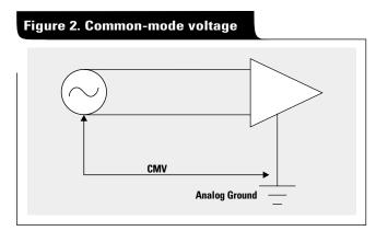
effects can be intermittent reboots, lockups, and bad data transfer. Network interface cards, serial ports, parallel ports, and modems are prime targets for some form of failure due to high CMV. If the CMV is high enough, component failure is possible.
