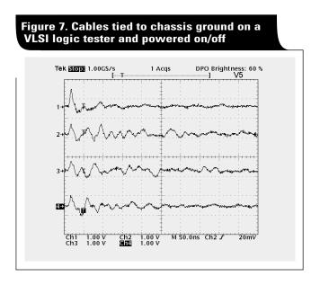
out that if the same test were done today, the results would be different because the noise level varies constantly. The noise was very unpredictable in all cases. We will never be able to eliminate all the noise in our environment. A good defense for common-mode noise would be to choose components that have a very high CMRR and a high commonmode operating range, such as the Texas Instruments LVDS and LVDM products.
