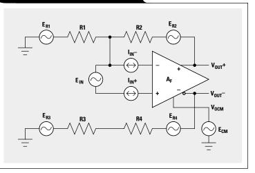
$E_{OD}$  is the differential RMS output noise voltage.  $E_{OD} = A(E_{ID})$ , where  $E_{ID}$  is the input noise source, and A is the gain from the source to the output. Half of  $E_{OD}$  is attributed to the positive output (+ $E_{OD}/2$ ), and half is attributed to the negative output (- $E_{OD}/2$ ). Therefore, (+ $E_{OD}/2$ ) and (- $E_{OD}/2$ ) are correlated to one another and to the input source, and can be directly added together; i.e.,
