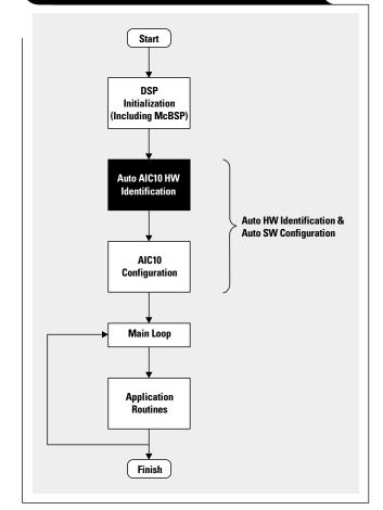
Otherwise the auto-identification failure flag (IdentFail) is set, a warning message is displayed, or an alarm sounds, aborting the system to reset condition.
