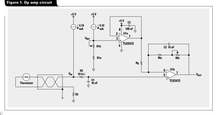
One of the two current regulators supplies 100  $\mu$ A  $\pm 0.5\%$  to the thermistor. From resistance and current information, the thermistor voltage is 0.06783 V for 100°C and 3.265 V for 0°C.
