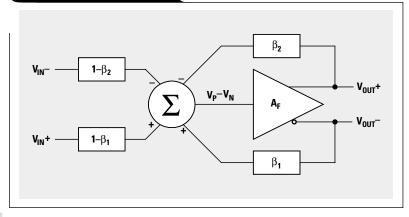
diagram from which specific circuit configurations can be easily solved. The voltage definitions are required to arrive at practical solutions.
