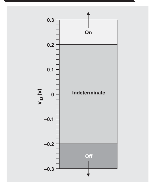
Figure 4. RS-485 differential voltage states
