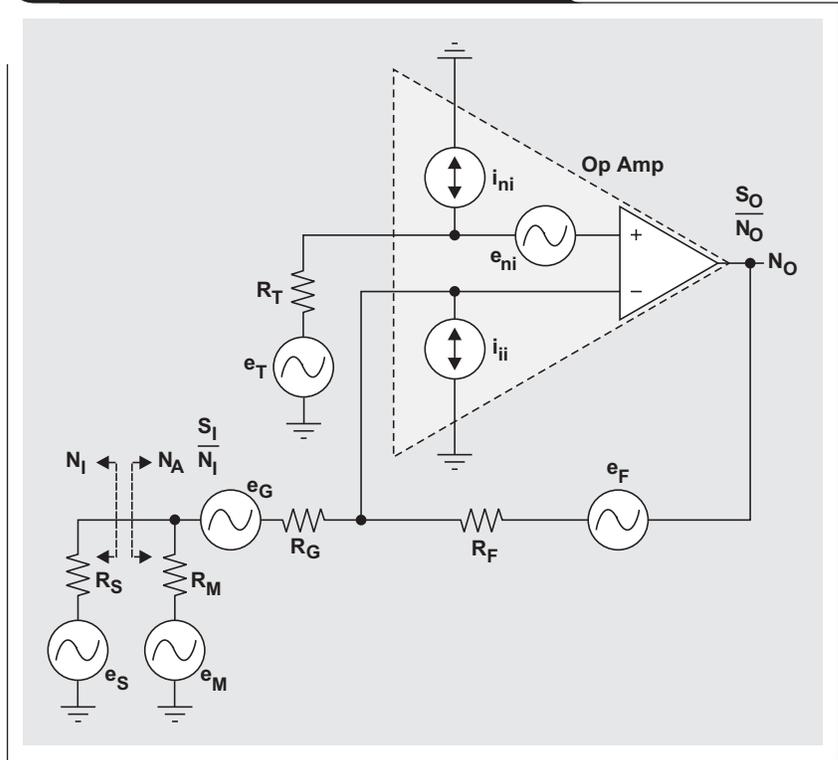
Figure 3. Fully differential noise analysis diagram
