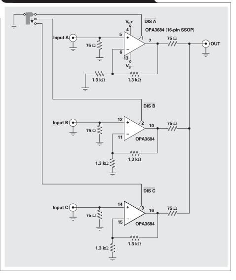
Figure 2. Video switcher with high-speed op amps
