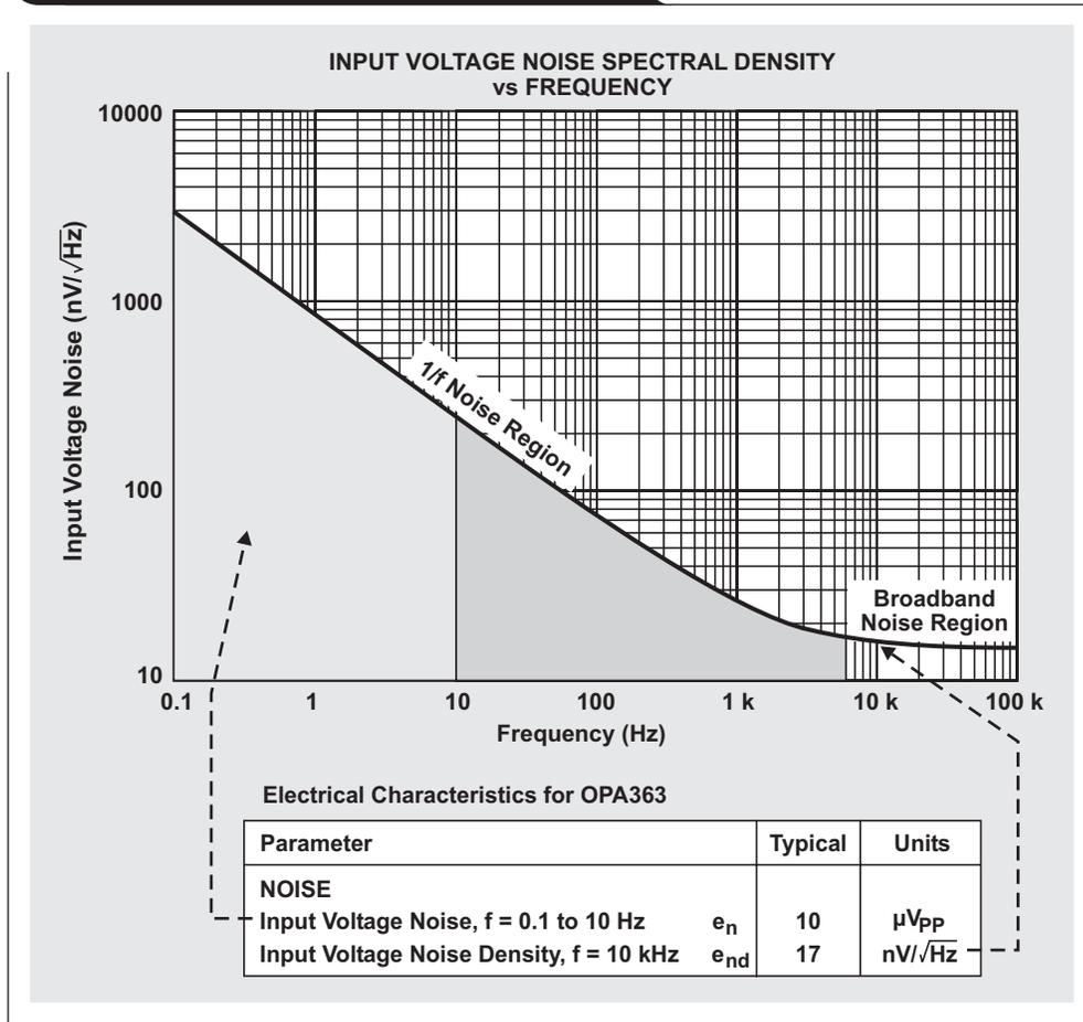
and input voltage noise density specifications (see Figure 2). The input voltage noise specification ( $10 \mu\text{V}_{PP}$ ) describes the low-frequency noise of the amplifier in terms of a bandwidth. This bandwidth is part of the 1/f noise region of the amplifier. The transistors in the input stage of the amplifier, along with the input-stage active load, generate this noise.
