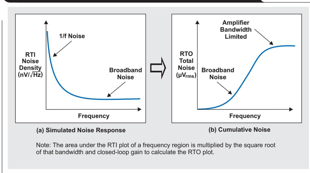
contribution is low. In region  $e_2$ , the broadband noise of the amplifier is multiplied by the amplifier circuit gain, which is again +1 V/V, and the square root of the bandwidth.
