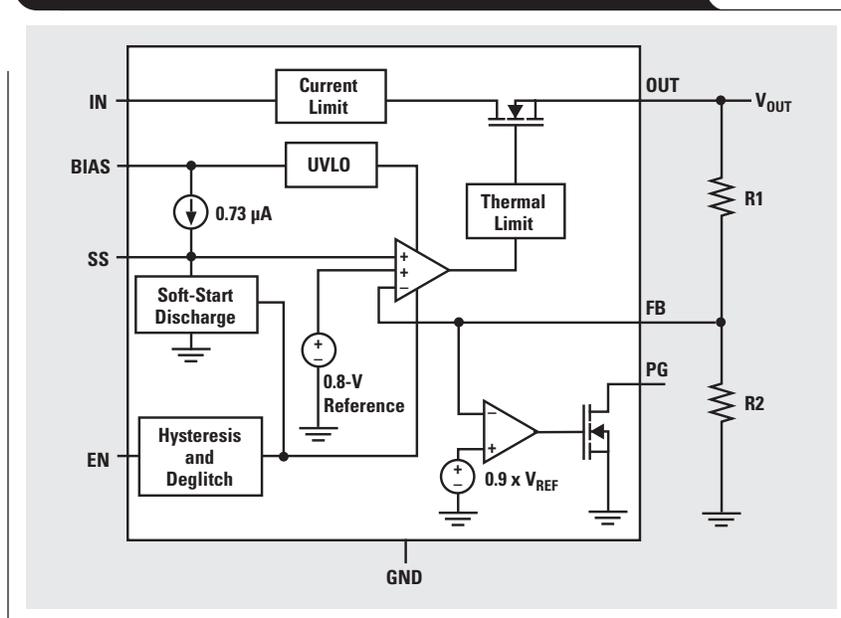
internal circuits run off the higher BIAS input, the device is capable of achieving regulation from a low-voltage input supply. In fact, the power input,  $I_{IN}$ , is limited only by the output voltage and dropout of the device.
