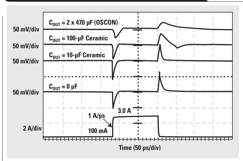
resistance (ESR). Using a patented feedback control topology, the TPS74x01 family, configured with  $V_{BIAS} = 3.3 \text{ V}$ ,  $V_{IN} = 1.8 \text{ V}$  and  $V_{OUT} = 1.5 \text{ V}$ , achieves fast transient response times (see Figure 2) with no output capacitors but is still stable with larger capacitors having ESR. The absence of output voltage ringing after the load transient shows that the regulator is very stable with no output capacitance.
