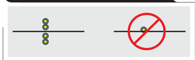
Figure 18. Avoiding via clearance sections
