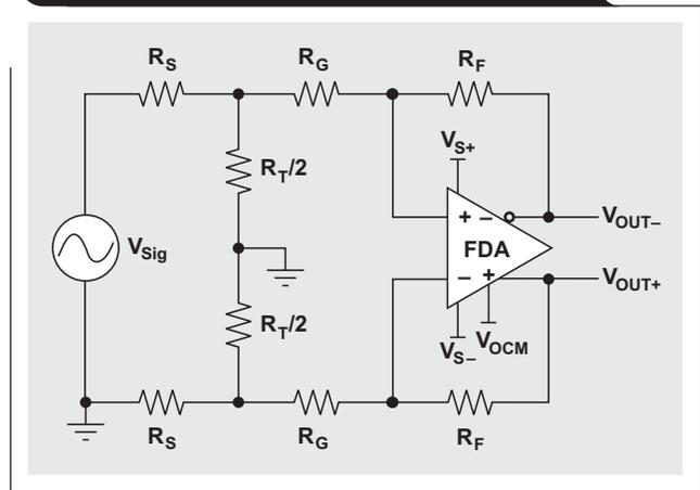
Figure 6. Equivalent SE bipolar input circuit
