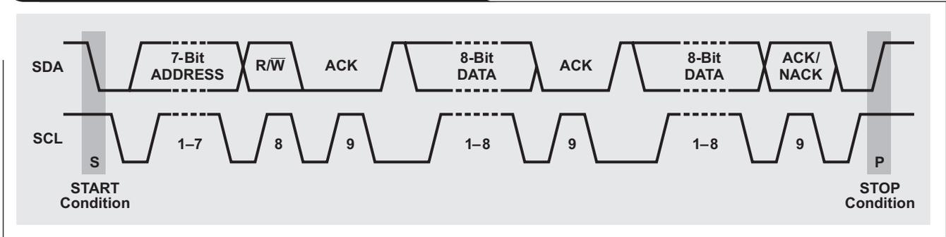
The bus has two roles for nodes: master and slave. A master issues the clock and slave addresses and also initiates and ends data transactions. A slave receives the clock and addresses and responds to requests from the master. Figure 2 shows a typical data transfer between master and slave.
