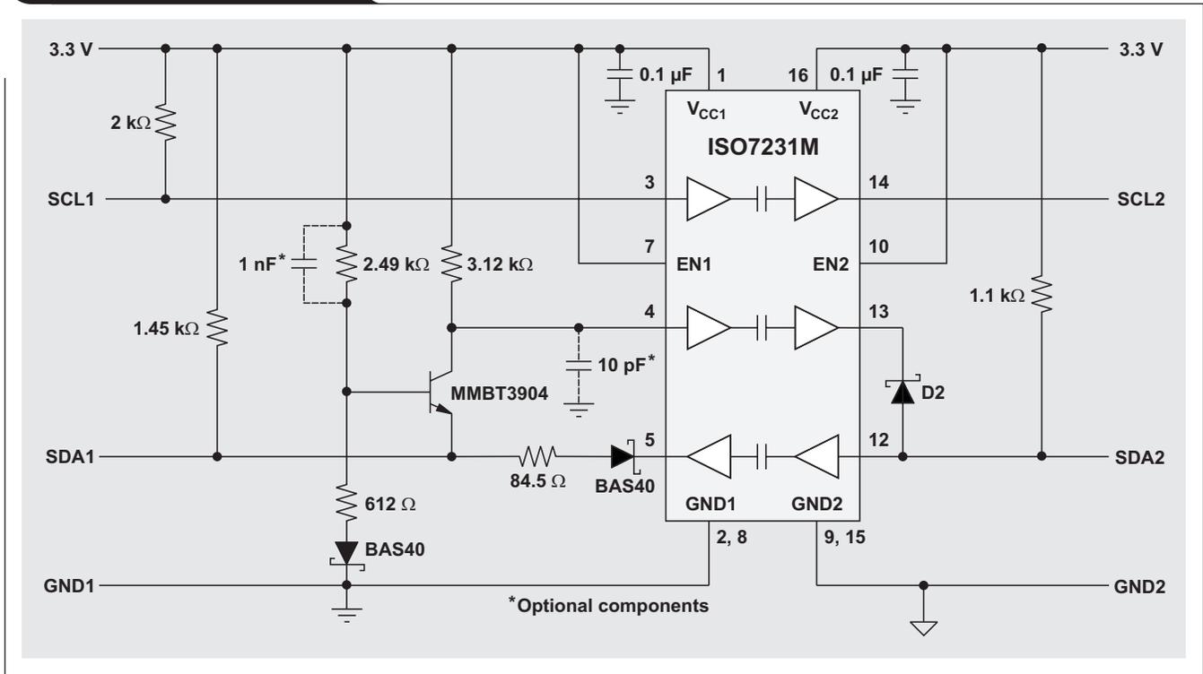
Figure 5 shows the final isolator circuit for the majority of I<sup>2</sup>C applications where the master is isolated from a slave bus. In this case, only the SDA line is bidirectional, while the SCL is unidirectional. For a multi-master system in which both lines must be bidirectional, the SDA circuit design can also be applied to the SCL when an ISO7242M isolator is used.
