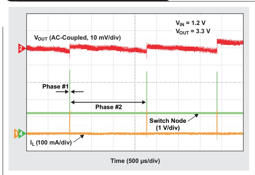
**Figure 3. Switching pulse of TPS61220 during no-load operation**
