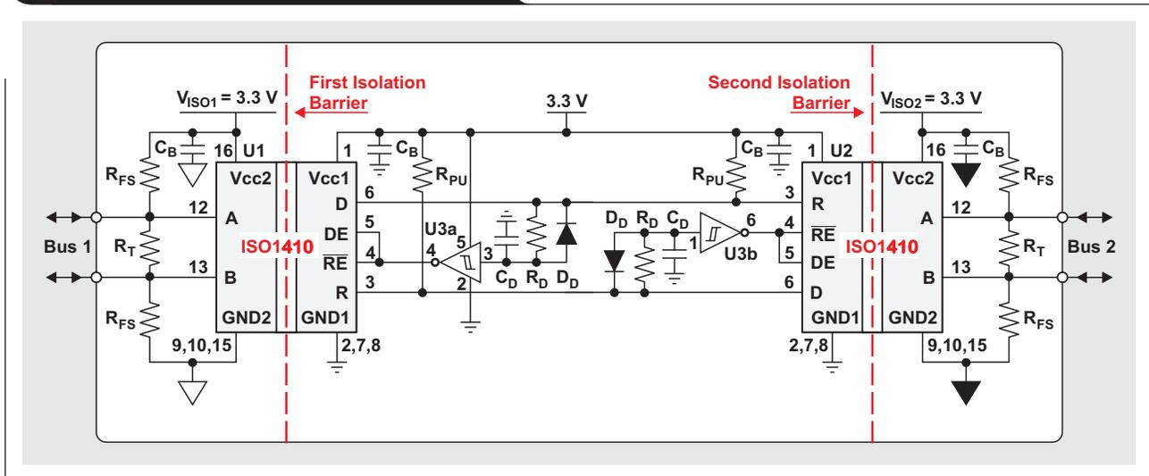
**Figure 6. Design for dual isolated power supplies**
