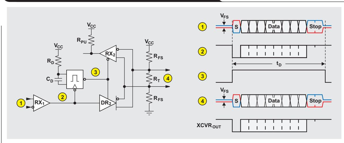
**Figure 4. Transceiver timing control with an inverting buffer**
