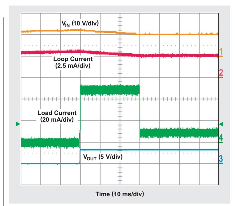
Finally, the energy-harnessing power supply stores enough energy in the bulk capacitor and operates over a wide enough input-voltage range to supply continuous pulses of power to the load. Figure 5 shows the supply providing 20 mA to the load for a duration of 100 ms every second, with the supply's output voltage remaining regulated.
