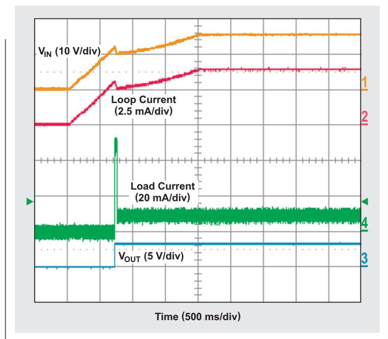
**Figure 4. Energy-harnessing power supply providing load's start-up current**
