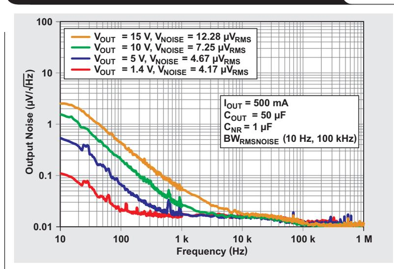
**Figure 5. Excerpt from TPS7A4700 datasheet showing integrated output noise voltage**
