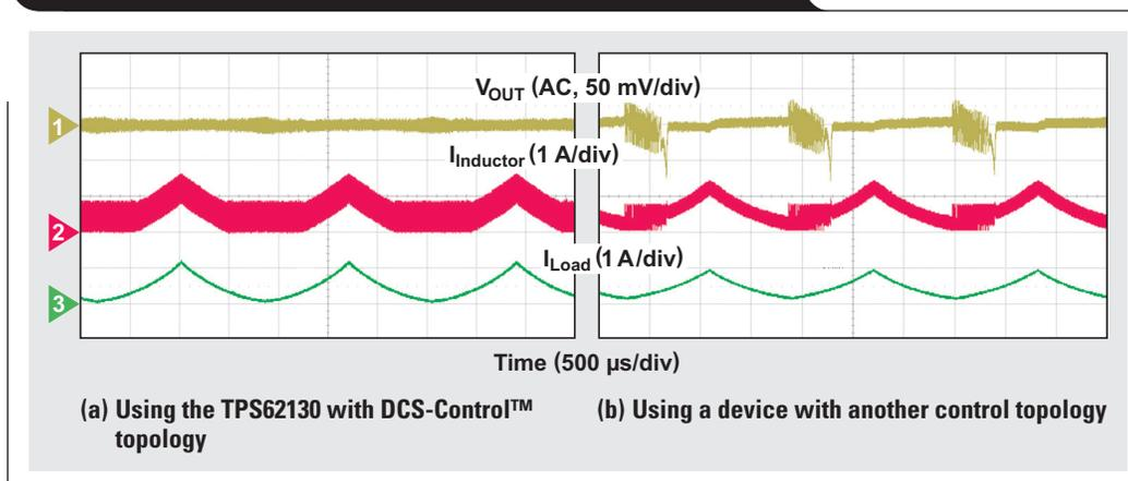
start of the transient and when the high-side MOSFET turns on means that the transient response is limited almost entirely by large-signal concerns (the inductance) and not by small-signal concerns (the control topology). Thus, the DCS-Control topology is not the main limitation of the transient-response capabilities of the device; rather, it enables outstanding transient response for given output-filter components.
