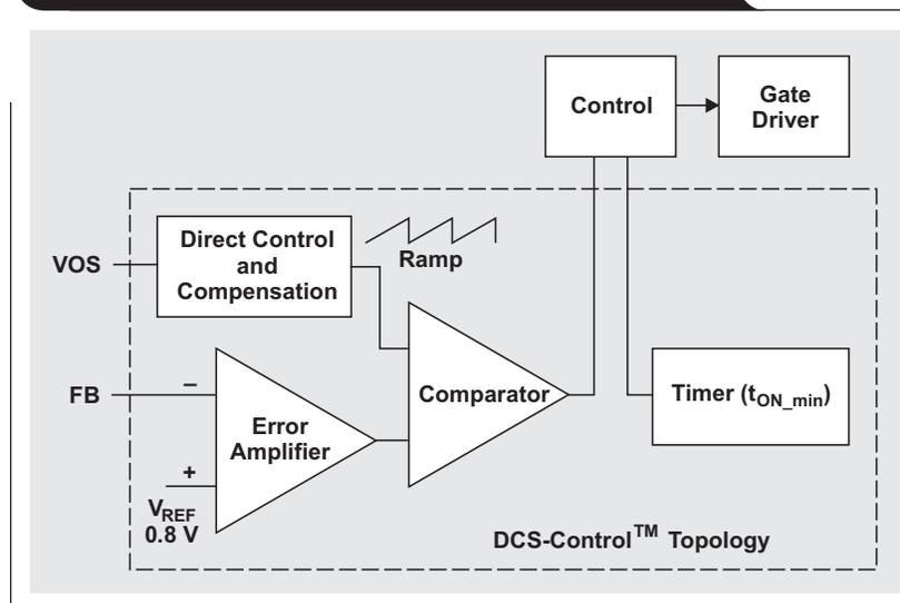
The comparator then outputs a signal to the control circuit, telling it whether or not to output a switching pulse to the gate driver, which controls the high-side MOSFET. The comparator works with the timer circuit to provide both the fastest response to load transients and a regulated switching frequency.
