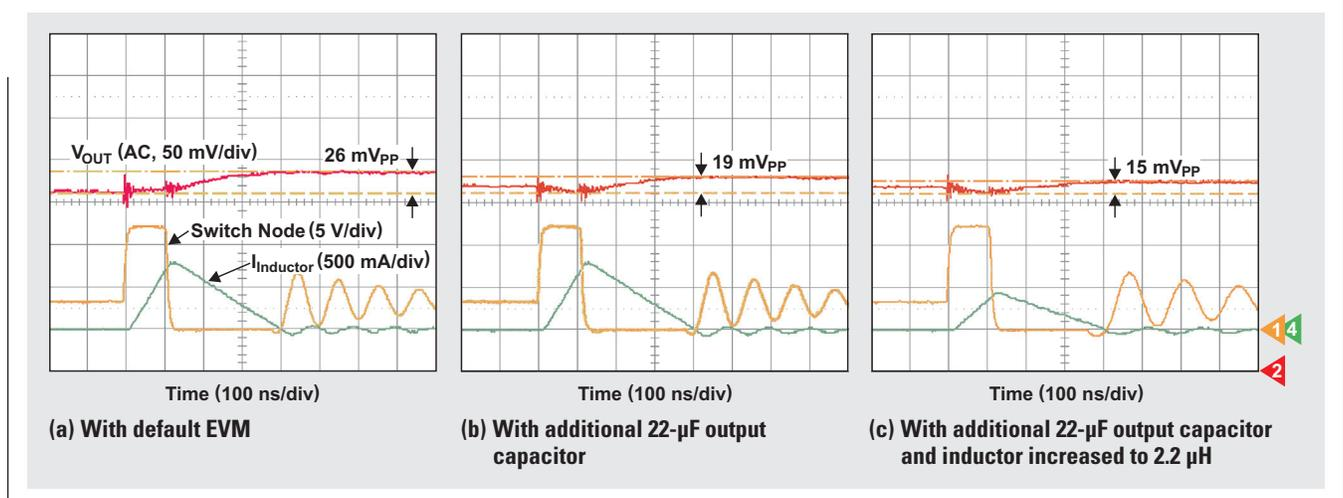
requirements. As an example, consider the output-voltage ripple in the power-save mode of a system with a 12-V input and 3.3-V output. TI's TPS62130 evaluation module (EVM),<sup>4</sup> operating at the 2.5-MHz setting, was used for Figure 2 to demonstrate how to decrease the ripple by increasing the external inductance and output capacitance. The no-load condition was used to show the worst-case output-voltage ripple in power-save mode.
