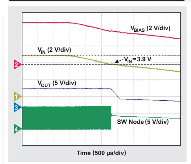
**Figure 4. Split-rail approach feeding  $V_{OUT}$  back as bias supply**
