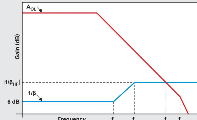
**(b) Open-loop gain and inverse feedback factor**
