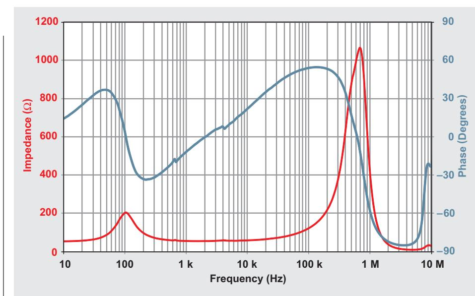
Two resonant peaks are clearly evident in the impedance plot. The low-frequency resonance at 100 Hz is produced by the mechanical and electrical properties of the drivers in the headphones. The high-frequency resonance is created from the interaction of the cable
