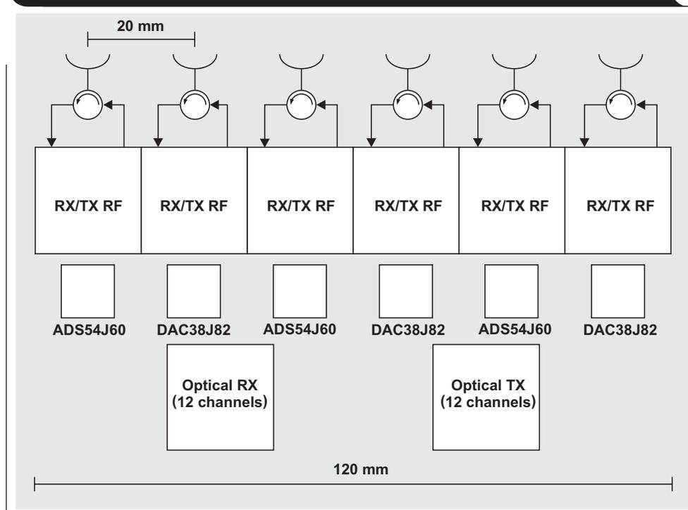
**Figure 3. High-level phased-array radar system diagram using optical fiber in the JESD204B link**
