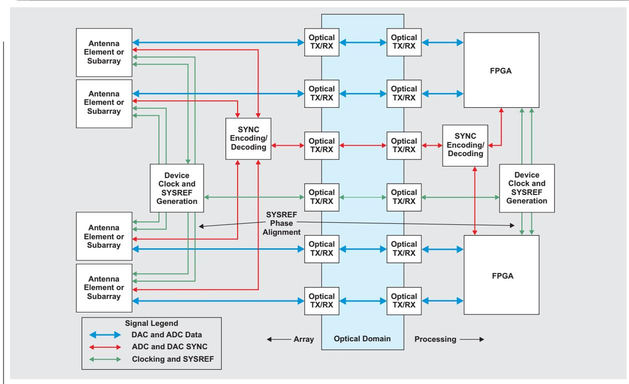
uses SYNC signal aggregation. A designer can do this by ANDing signals together to limit the total number of SYNC signals transmitted over the optical link. Note that SYNC can have timing requirements for subclass 1 implementations when numerically-controlled oscillators (NCOs) are used as part of digital up or down converters within the data converters.<sup>[3]</sup>
