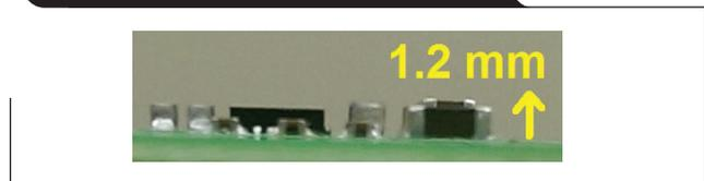
low-profile applications require a maximum height that is less than 2.5 mm, which precludes this converter from being used.
