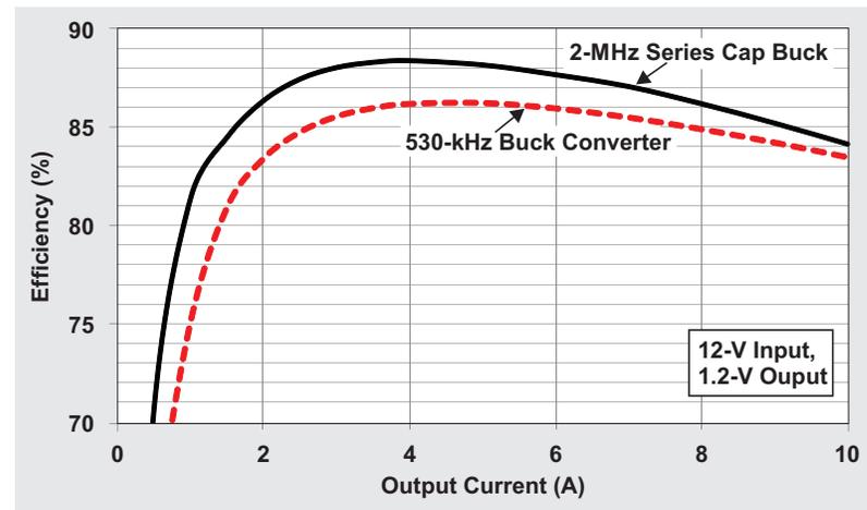
**Figure 8. Efficiency comparison with different inductor sizes**
