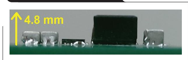
**Figure 6. Side profile of a series-capacitor buck converter**
