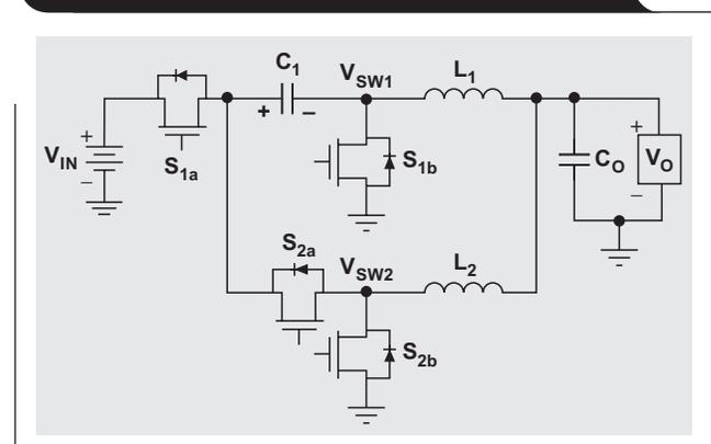
**Figure 3. Conventional buck converter requires 264-mm<sup>2</sup> board area**
