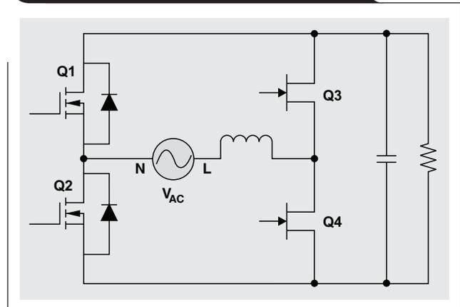
peripherals, is a good candidate for this topology. Even though the traditional control method cannot be directly applied to a totem-pole PFC, special control algorithms need to be developed. In fact, the control of a totem-pole PFC is much more complex when compared to a traditional PFC. Lacking a bridge rectifier, the bidirectional inductor current and the function swap between the main switch and the sync switch creates many challenges in a totem-pole PFC design.
